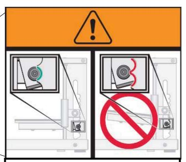
Carriage must be fully engaged before user board's platform. Users must be instructed how to adjust and secure the platform. Failure to properly engage platform could lead to injury.
